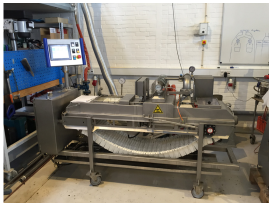
Ill. 3.3 Test equipment for SonoSteam treatments at FORCE Technology.
