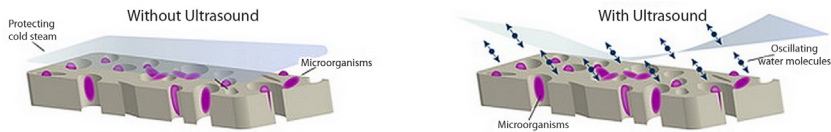
Fig. 3.4 Process of steam-based disinfection without and with ultrasound (FORCE Technology 2014) .
