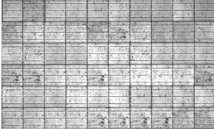
Figure A.1: Electroluminescence image of a crystalline silicon PV module measured at STC I_{mp} bias, taken before the module has sustained any mechanical damage.
