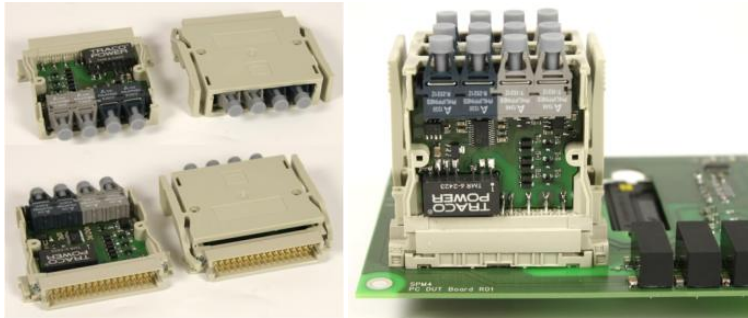
Fig. 2-8 Prototype of on-line V_{CE\_ON} and V_F measurement circuit using MOSFET for the power cycling test.
