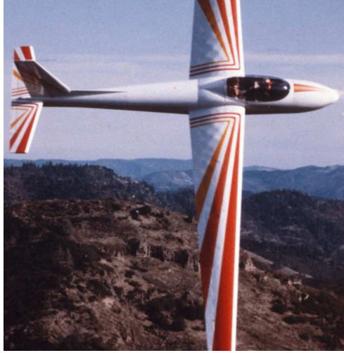
Figure 1.5: Glider plane making a tight turn. Clear buckles are present on the wings. Photograph courtesy of Connie Indrebo.
