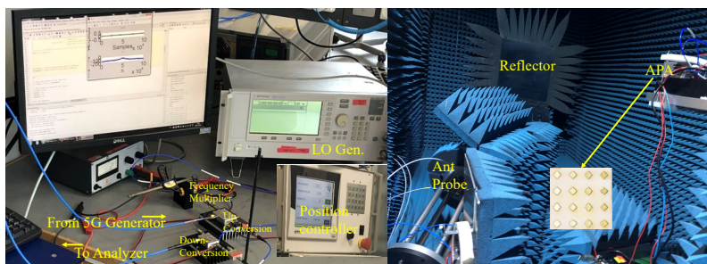
Fig. G.4: Measurement setup using compact antenna test range chamber.
