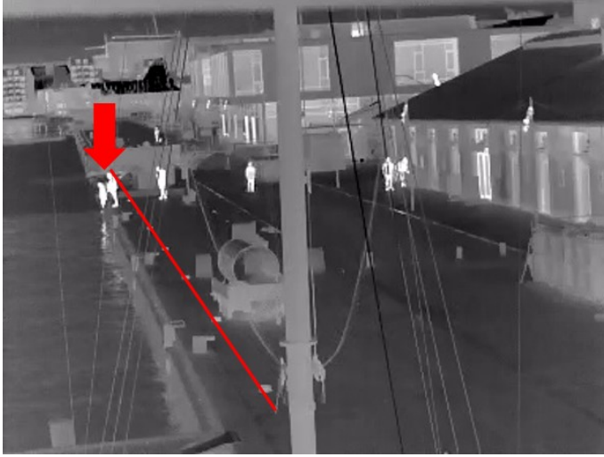
Fig. E.1: Thermal surveillance imaging for detecting potentially dangerous situations and alerting authorities. An alert should be raised when someone crosses the red line.
