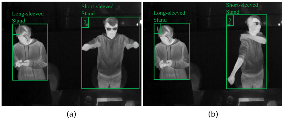
Fig. 2.10: How the tracking-by-detection module will result in for an input video. (a) and (b) are two frames from the video where ID numbers 1 and 2 indicate the two persons across frames, respectively. At the same time, each person's clothes type and posture type are recognized by the classification header of YOLOv5. Adapted from [6].
