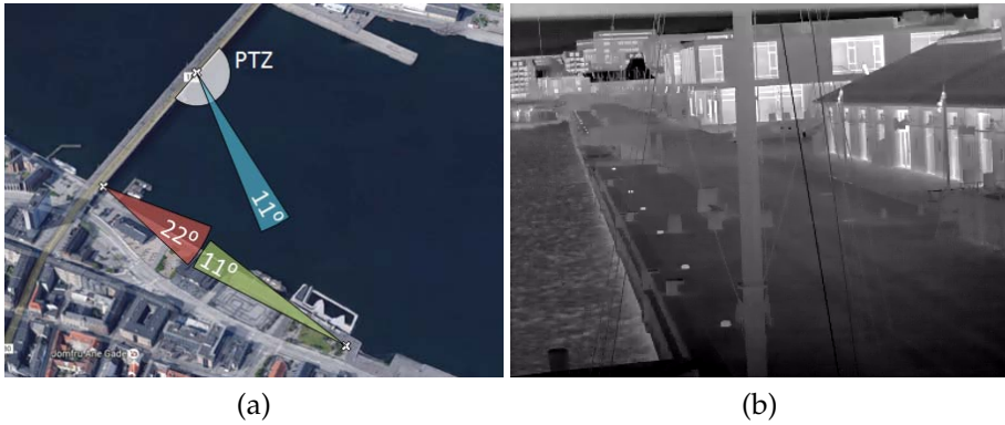
Fig. 3.1: The specific region under monitoring by the surveillance system with three cameras is shown in (a). An thermal image acquired by the camera with a FOV of 22^\circ is shown in (b). Image source: (a) [8].
