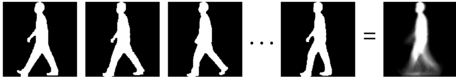
Fig. D.2: Human silhouettes in a gait cycle and the averaged gait energy image (the right one) for gender classification. Image source: [16].
