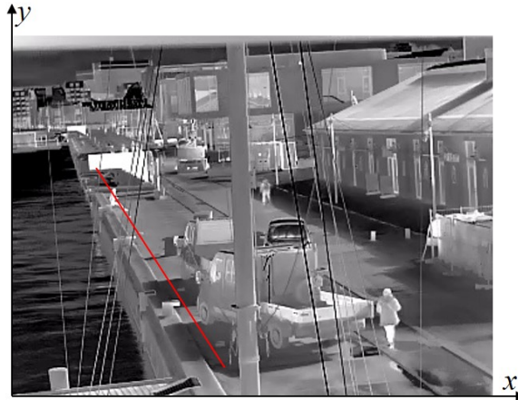
Fig. 3.7: The red line indicates the alarm boundary and the left of it is defined as the alarm region. Image source: [37].
