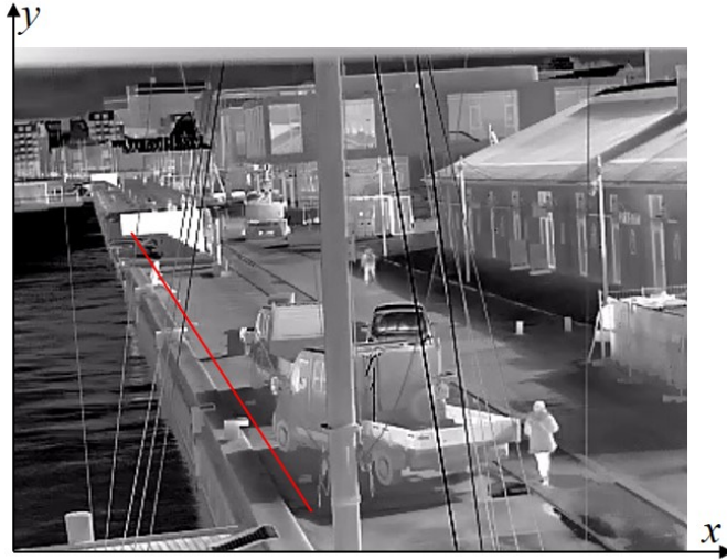
Fig. E.4: Alarm region defined as the area between the red line and the water.
