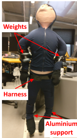
Fig. H.2: View of the created low-cost doll, together with clothes and ankle weights.
