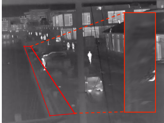
Fig. 3.8: The region from the water edge to the alarm line is defined as the input for the autoencoder to detect anomalies. To make the region rectangular, a transformation is then required. Image source: [37].
