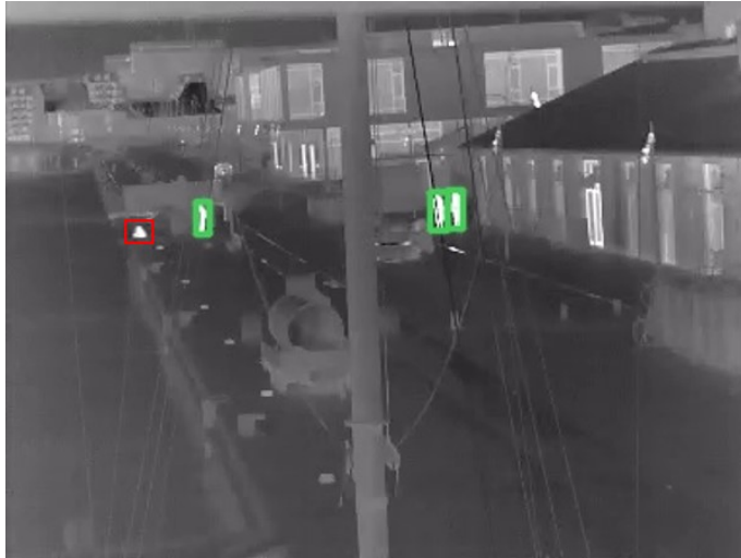
Fig. E.7: A failed case which should have raised an alarm. The red box refers to the undetected person.
