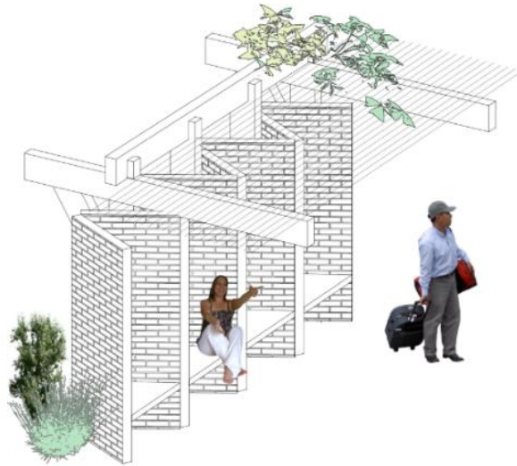
Figure 125. A bus stop made from the same waste materials. The wooden elements are used for canopy, while the folded brick walls are stabilized via the seating elements.
