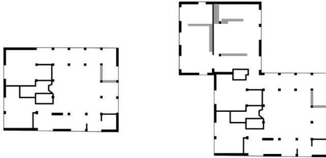
Figure 113. The original plan from 1961, and the house with the later extension in 1998. (Own redrawing)
