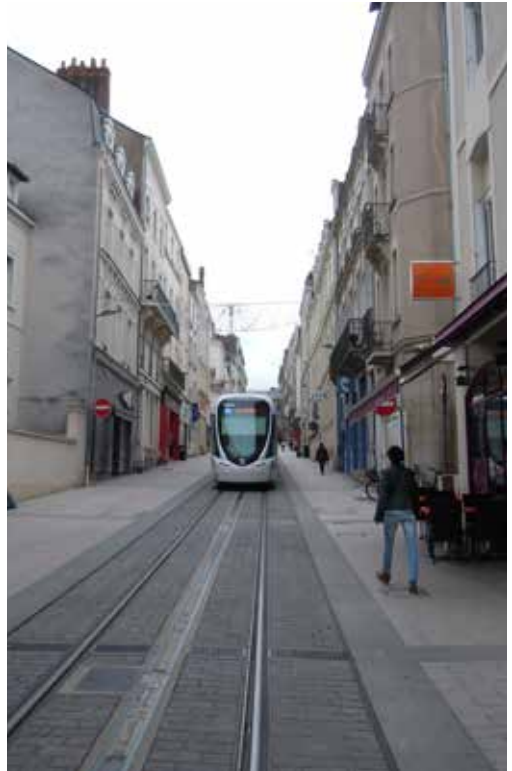
FIGURE 16: A special ground power supply APS is chosen in Angers, this is in order to limit the visual effects of overhead wires in the historical city centres. There are 700 m in Avrielle and 725 in Angers centre. Compared to a traditional over head power supply the additional prices for this system was 1,5 mio. Euro. (Photo by author).
