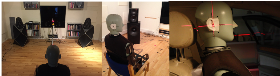
Fig. 10: In-situ measurements using a dummy head in ordinary rooms and car cabins.
