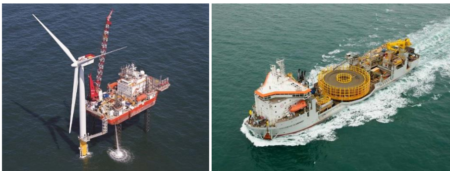
Figure 1-16 Example of support vessels: jack-up barge in left and cable laying vessel in right (offshorewind.biz)
