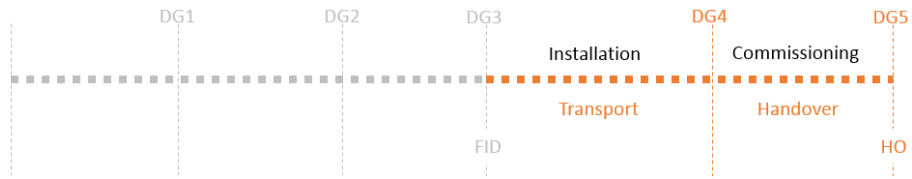
Figure 1-6 Breakdown of construction phase of an offshore wind project
