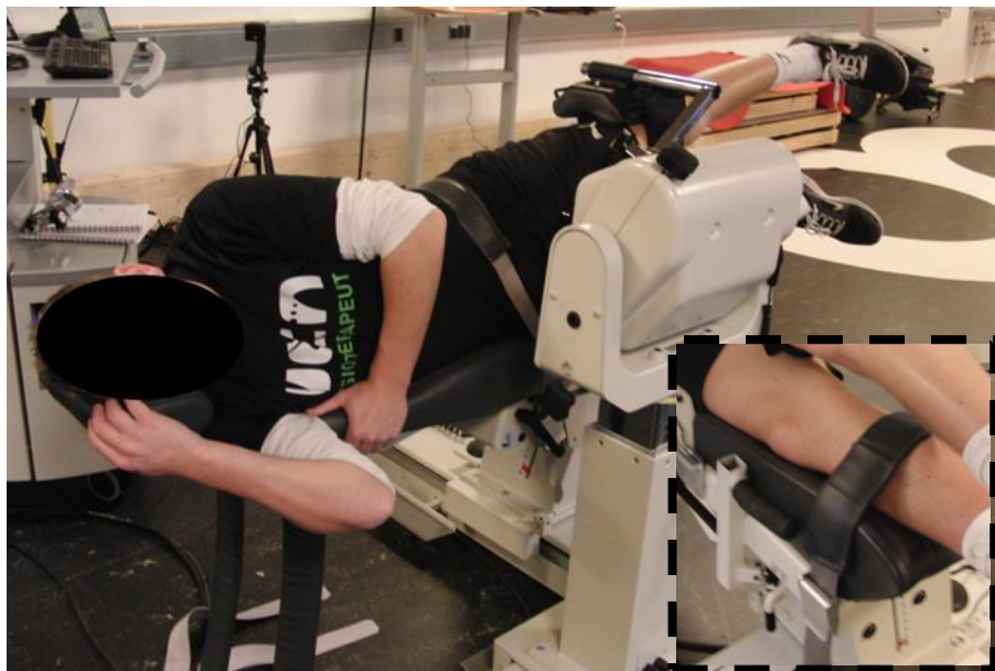
Figure 6: The body position in the Biodex dynamometer just before the start of a measurement of eccentric hip abduction strength.
