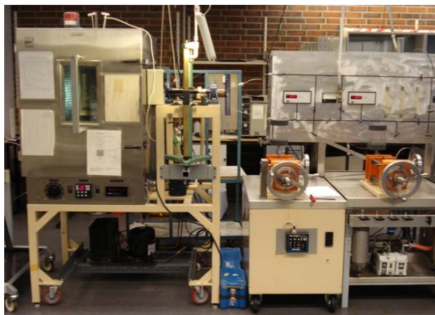
Fig. 4.3(a and b) An Actual photograph and Schematic diagram of JEFRI-DBR PVT system
