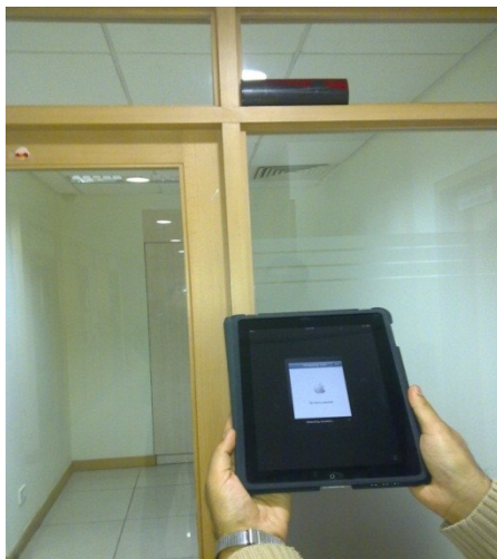
Figure 7-8 Cognitive UAB modem implemented on Apple iPad receives location messages transmitted by a UAB transmitter (an mp3 player is used) kept at the top.
