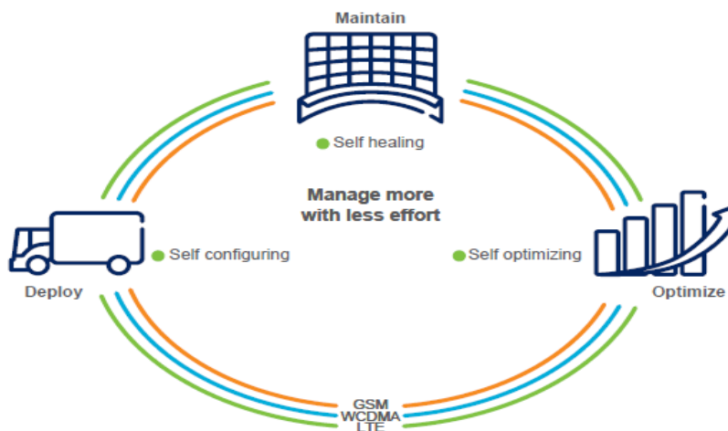
Figure 1.2 SON functionality across all technologies (Source: Ericsson)
