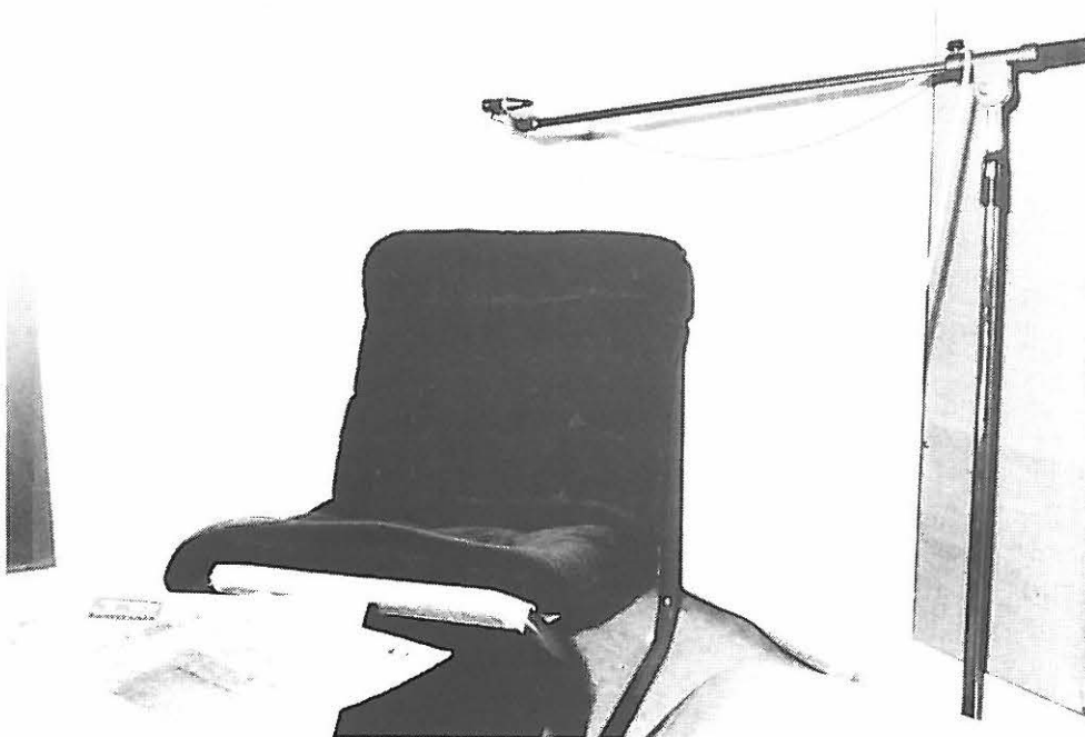
Measurement of the sound field at the position of the subjects head.
