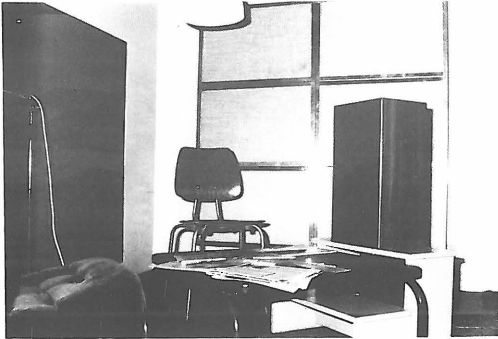
The test chamber with the easy-chair (extreme left), infrasound loudspeakers behind the cloth (back-left), newspaper at the table and audiosound loudspeaker (right).
