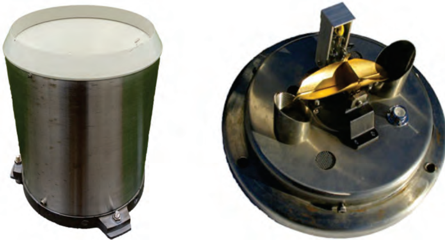
Figure 3: A Rimco 7499020 tipping bucket rain gauge shown in closed and open state. The last three digits of the model name defines the tipping bucket size, corresponding to 0.2 mm precipitation pr. tip.
