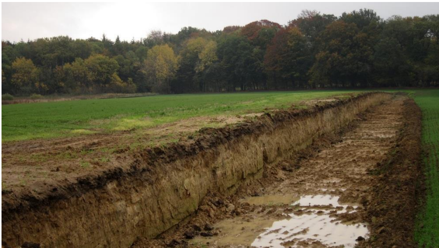
Figure 3.3: A clay pit for production of red bricks. The top-layer of the clay deposit is removed, after which the site is restored to its original purpose. Photo: Morten Bidstrup.
