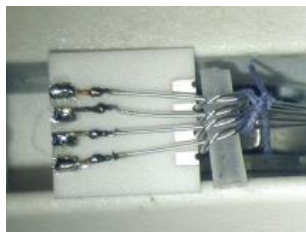
(c) Knots for wire tension relief
