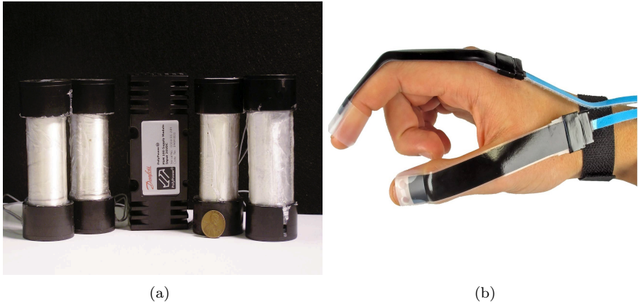
Figure 1.2: Illustration of (a) Danfoss PolyPower ® A/S push InLactor ® actuators with end caps and electrical connections (b) StretchSense ™ versatile wireless stretch sensor installed on a human hand.
