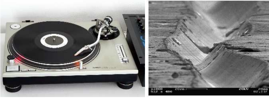
Fig. 3.2: Left: a turntable historically considered appropriate for DJ sets, Technics SL-1200 (ref. [53]); right: electron micrograph of phonograph vinyl record grooves (ref. [57])
