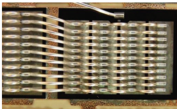
Fig. 3-4: IGBT B before painting (left) and after painting (right)
