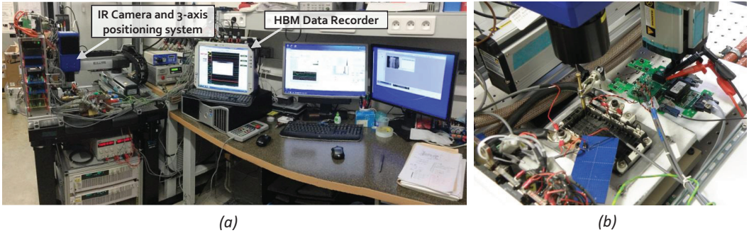
Fig. 3-5: (a) Panoramic view of test bench (b) Close up of power module, IR Camera, and gate driver with peak detector measurement circuit
