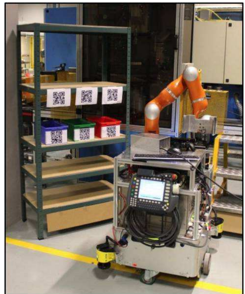
Figure 8 The Station 4 warehouse shelf system for finished SQFlex rotors. The shelf system has capacity for both SLCs containing finished rotors and empty SLCs for Station 3. LH2 handles the logistical challenge of SLC handling between workstations
