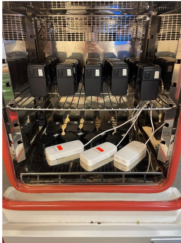
Figure 4: IEQ sensors (black sensors) and IC meters (white sensors) placed in the environmental chamber.
