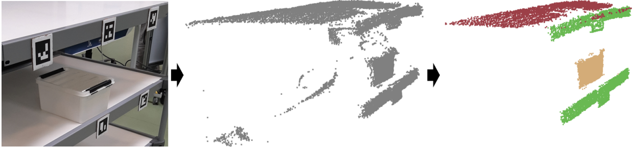
Fig. 2. Iterative execution of RANSAC and removal of inliers can segment a large point cloud, such as that seen in the middle, into smaller planes, such as those seen to the right, while also removing overall noise.
