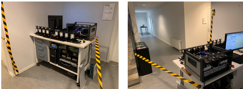
Fig. 2.22: Picture of the multiple-antenna setup and the perfectly reflecting sample (gold mirror) located 10 m away.
