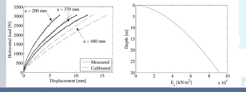
Comparison of numerical simulations with the Winkler model approach
