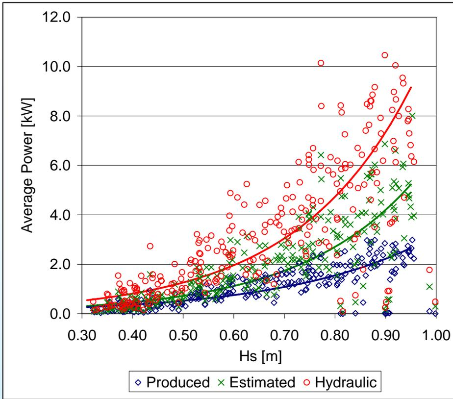
Optimal working point where  $Rc/Hs \approx 0.7$  not 1.0 as shown.
