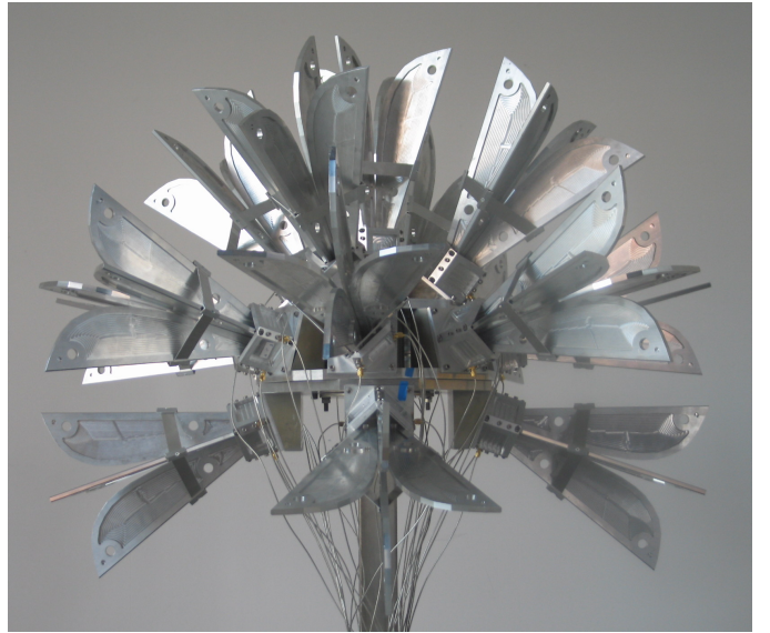
Fig. 5. The quad-ridged horn antennas in the spherical array arrangement.
