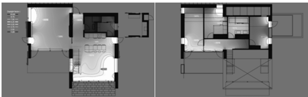
Fig. 2. Calculated daylight factor iso contours for ground floor (left) and upper floor (right).
