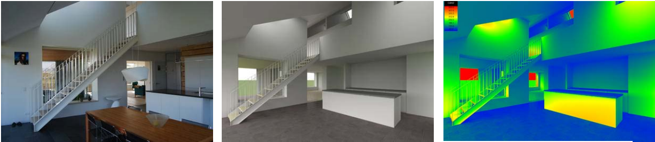
Fig. 4 One photo and two simulations of the luminance distribution made in VELUX Daylight Visualizer [5]. Photo by Gitte Gylling.
