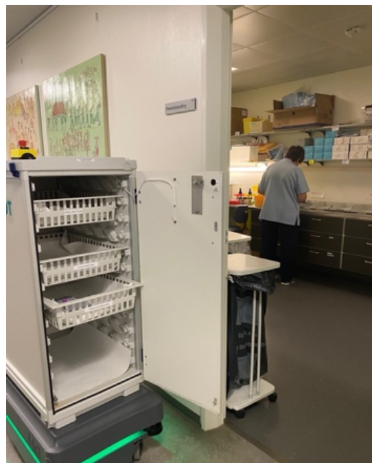
Figure 32 A look inside Hubot while the robot is waiting in the hallway for a MLT to load samples into its baskets
