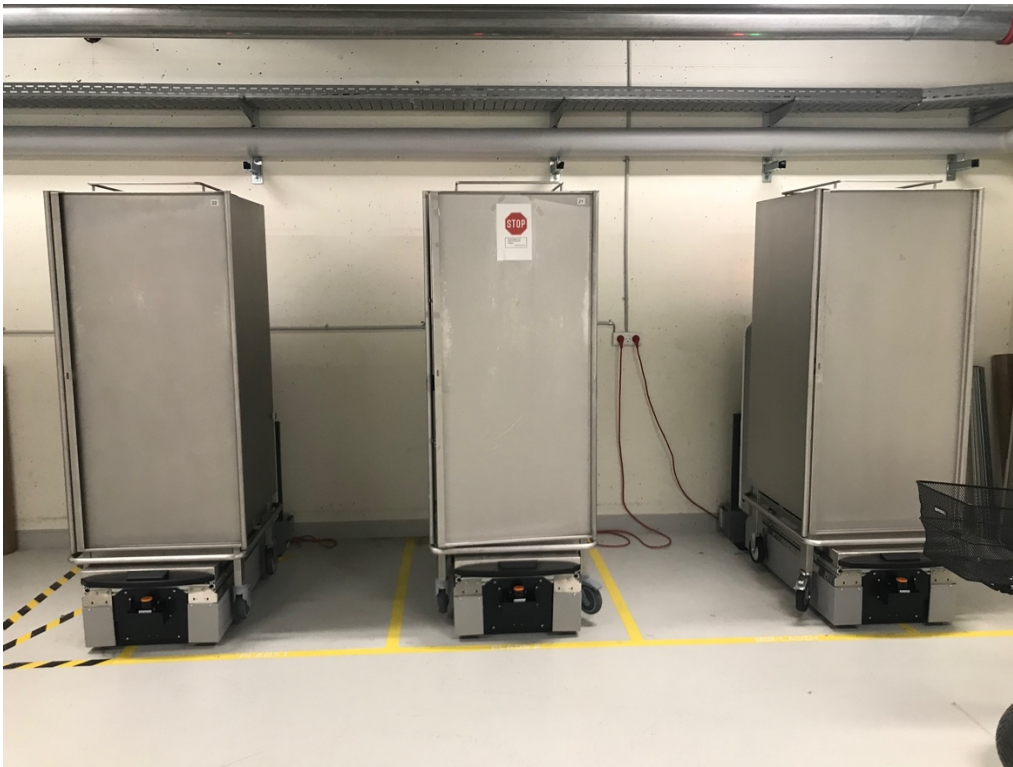
Figure 26 Mobile robots standing in docks at the hospital basement at SHS Aabenraa
