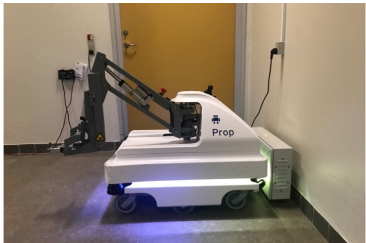
Figure 7 One of the robots, Prop, recharging in the dock in the Robot Garage in SHS Sønderborg
