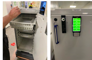
Figure 2. Left: A look inside Hubots' cabinet. Right: The handle, lock and smartphone attached to Hubot
