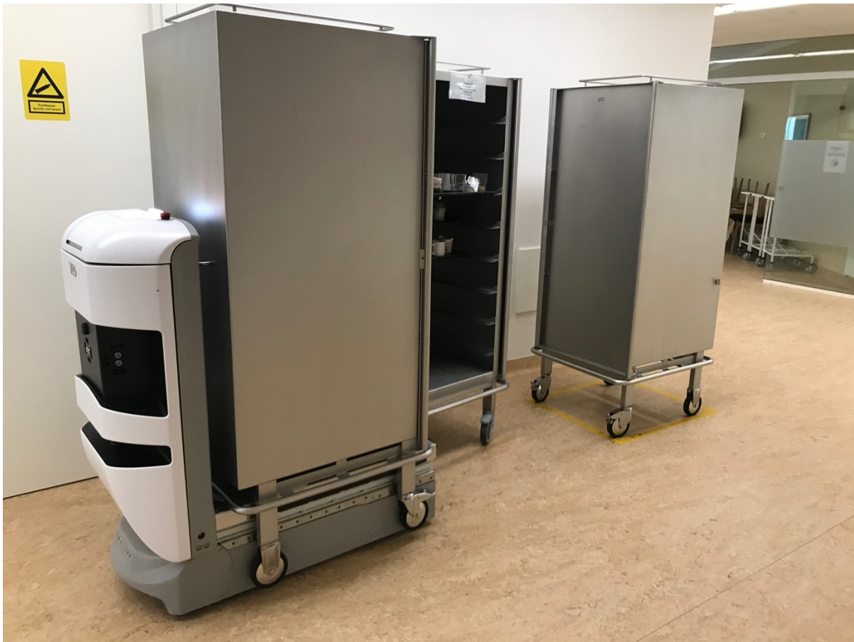
Figure 29 Mobile robot loaded with cart on hospital hallway at SHS Aabenraa
