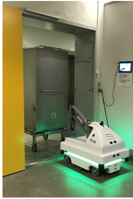
Figure 1: A MiR Hook 100 robot with a hospital kitchen service cart attached
