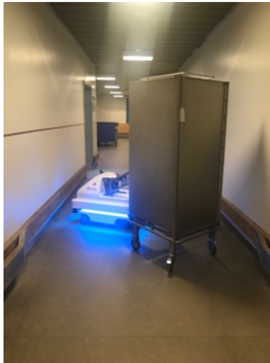
Figure 22 Mobile robot with cart attached, taking up space in the hallway at SHS Sønderborg
