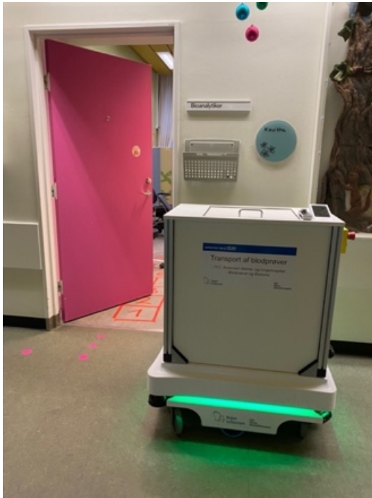
Figure 33 Hubot2 waiting in the hallway box to be loaded with blood samples
