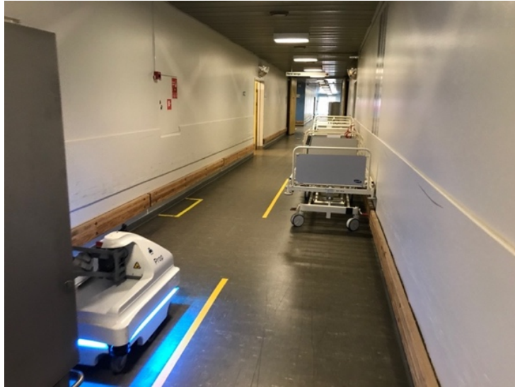
Figure 9 Robot with cart attached driving the narrow hospital hallways at SHS Sønderborg
