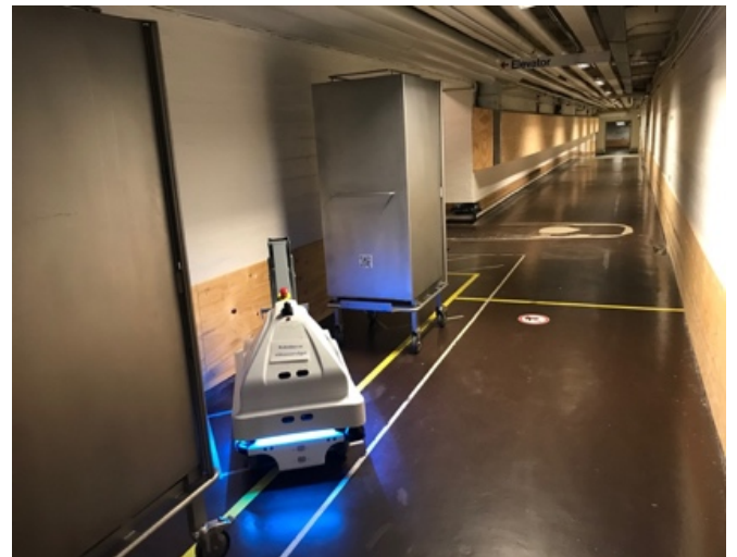
Figure 13 Robot placing carts in Robot placing carts in the hallways at SHS Sønderborg
