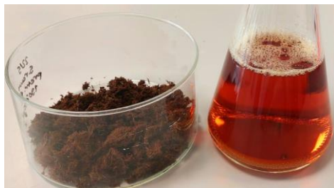
Figure 20 Salicornia ramosissima fibres and pretreatment liquid obtained from hydrothermal treatment of extractives-free fibres at 190 °C for 10 min (SF 3.7).
