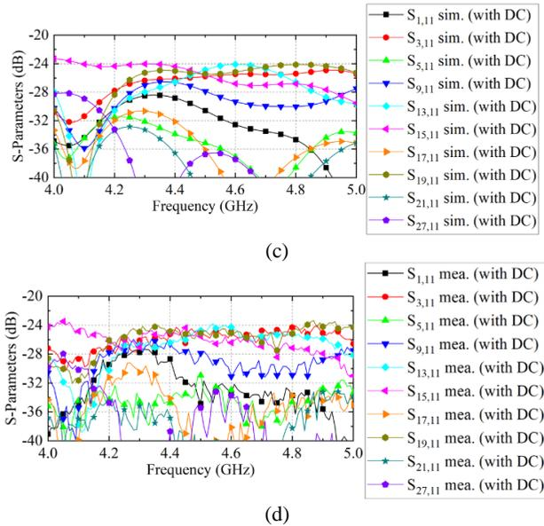
Fig. 3. The simulated and the measured S-parameters of arrays with and without DC: (a)  $S_{11,11}$  and  $S_{12,11}$ , (b) Simulated S-parameters of the array without DC, (c) Simulated S-parameters of the array with DC, (d) Measured S-parameters of the array with DC.
