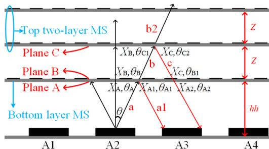
Fig. 1. The decoupling schematics of the TMS.
