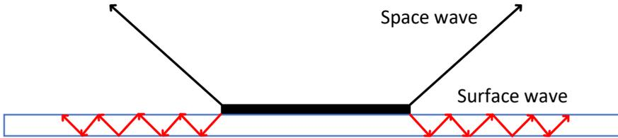
Fig. 2.3. Classical microstrip antenna model.
