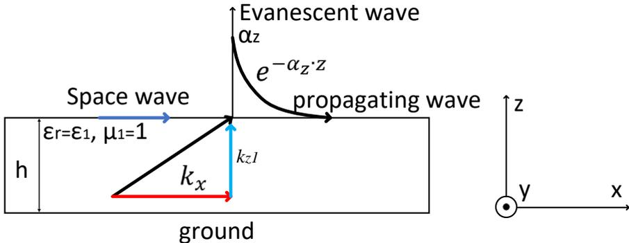
Fig. 2.4. The grounded dielectric slab waveguide model.
