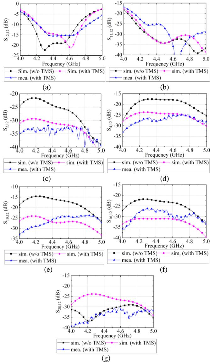
Fig. 9. The simulated and measured S parameters of the  $4 \times 4$  array with/without TMS: (a)  $S_{12,12}$ , (b)  $S_{11,12}$ , (c)  $S_{2,12}$ , (d)  $S_{4,12}$ , (e)  $S_{10,12}$ , (f)  $S_{16,12}$  and (g)  $S_{16,12}$ .
