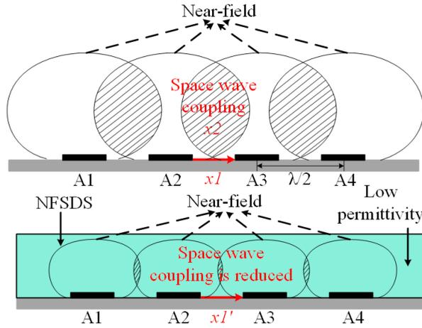
Fig. 1 The decoupling sketch of the NFSDS.
