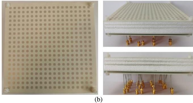
Fig. 8. The structure of the  $4 \times 4$  array with and without TMS: (a) the detailed structure of the array with TMS from top and side views, (b) the fabricated prototype of the array with TMS from top, side and perspective view.
