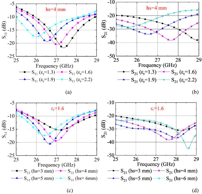
Fig.4 The S-parameters of the Array B with different  $\epsilon_r$  varying from 1.2 to 2.1 at a step of 0.3, and  $hs$  varying from 3 mm to 6 mm at a step of 1 mm: (a)  $S_{11}$  of the Array B with different  $\epsilon_r$  when  $hs$  is 4 mm, (b)  $S_{21}$  of the Array B with different  $\epsilon_r$  when  $hs$  is 4 mm, (c)  $S_{11}$  of the Array B with different  $hs$  when  $\epsilon_r$  is 1.6, (d)  $S_{21}$  of the Array B with different  $hs$  when  $\epsilon_r$  is 1.6.
