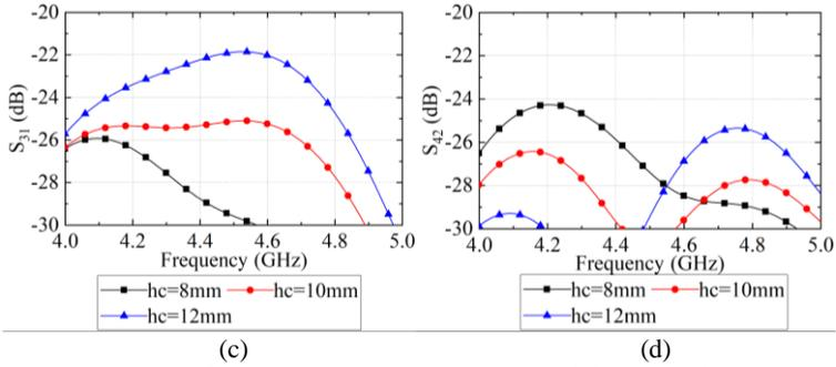
Fig. 7. The S-parameters of the arrays: (a) the S-parameters of the array with and without TMS in x-polarization, (b) the S-parameters of the array with and without TMS in y-polarization, (c) the  $S_{31}$  of the decoupled array with different  $hc$ , (d) the  $S_{42}$  of the decoupled array with different  $hc$ .
