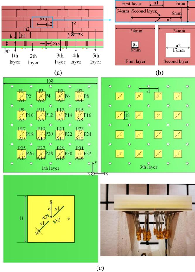
Fig. 2. Geometry and specific dimensions of the array with the proposed DC and the prototype: (a) the decoupled  $4 \times 4$  array, (b) the detailed structure and specific dimensions of the DC, (c) the reference array and the prototype.
