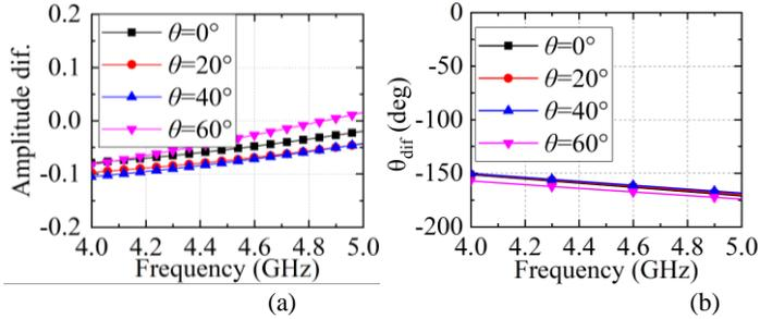
Fig. 5. The calculated amplitude difference  $A_{dif}$  and phase difference  $\theta_{dif}$  between the waves reflected from the bottom-layer MS the top two-layer MS when the incident angle of  $\theta$  varies from  $0^\circ$  to  $60^\circ$  with the step of  $20^\circ$ : (a) amplitude difference, (b) phase difference.
