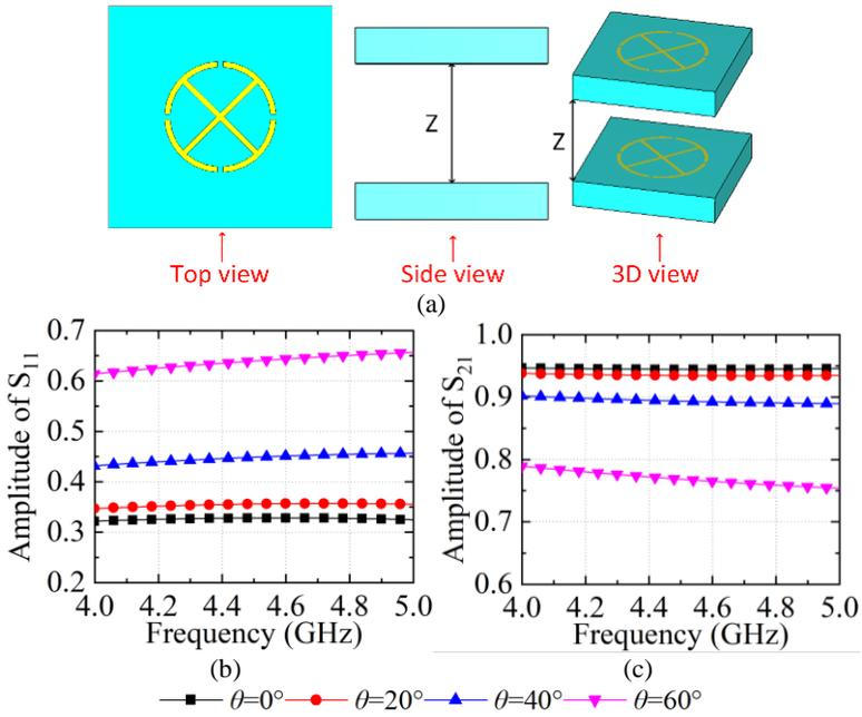
Fig. 4. Detail structure of the top two-layer MS, the amplitudes, and the phases of the S-Parameters of the top two-layer MS with different incident angle  $\theta$ : (a) the top two-layer MS, (b) the amplitude of the  $S_{11}$ , (c) the phase of the  $S_{11}$ .
