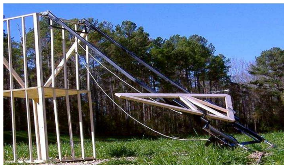
Figure 3: First year product developed to hoist residential trusses
