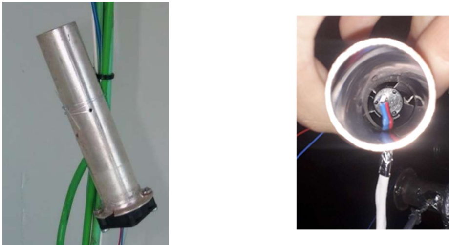
Figure 9: Pt100 temperature sensor placed in a mechanically-ventilated and silver-coated tube.
