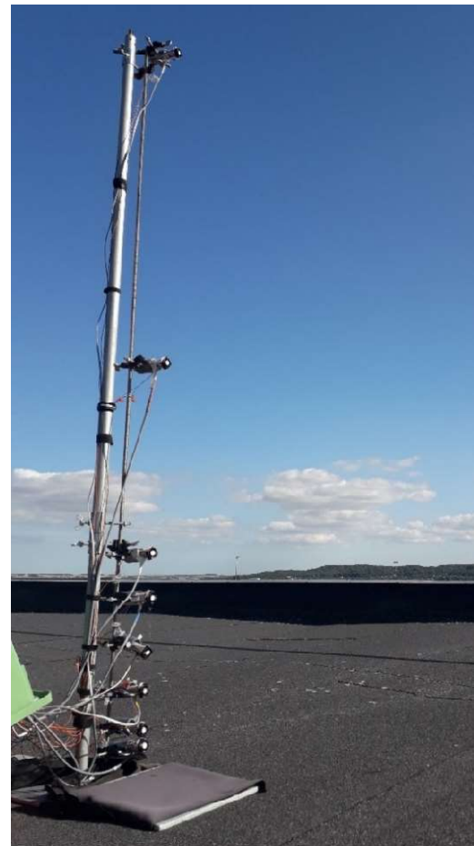
Figure 11: Air temperature measurement setup mounted on the roof of the building.
