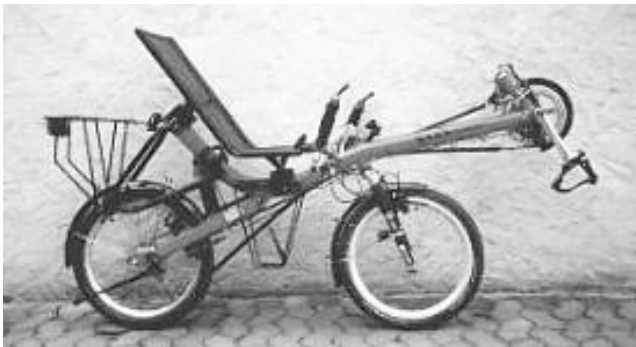
Figure 7: a contemporary recumbent bicycle 47
