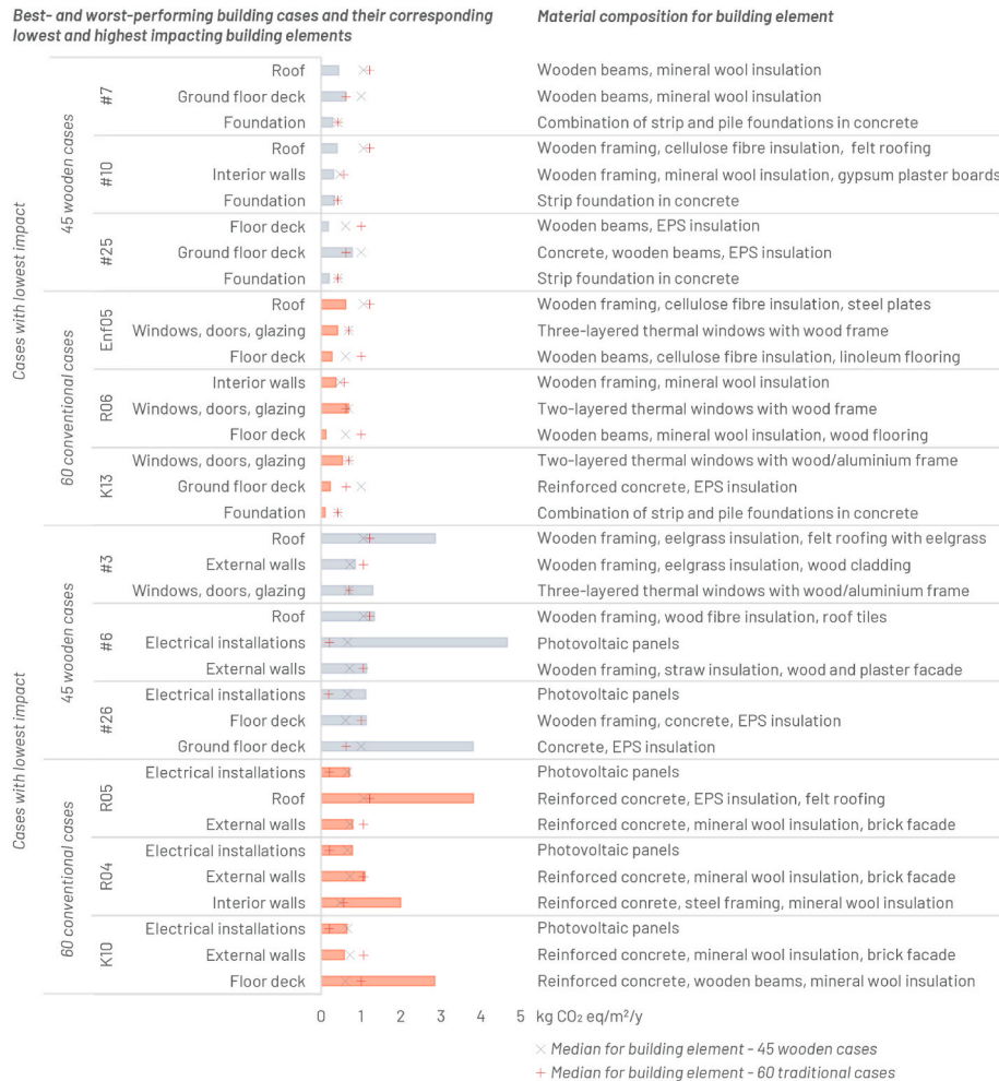
Fig. 9. GWP for the best- and worst-performing cases of the 45 wooden building cases and 60 conventional building cases [137] as well as material composition of the building elements.
