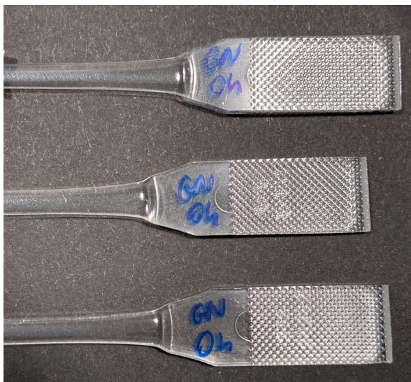
Figure S11. Photo-zoom of Figure S10 showing the neck reaching the thicker part of the tensile bar with a larger cross sectional area.
