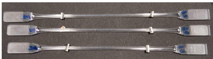
Figure S10. Photos of unaged poly(ethylene-co-1,4-cyclohexylenedimethylene terephthalate) (PECT) samples after creep tests at 30 °C with applied stress of 28.6 MPa for 24 h.
