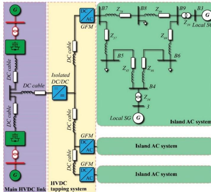
Figure 1 Illustration of the proposed HVDC tapping solution.
