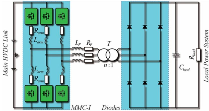
Figure 2 The topology of the proposed DC/DC tapping converter.
