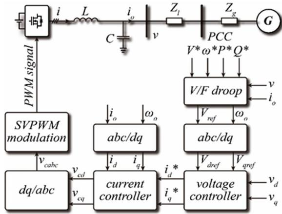
Figure 4 The topology and control block diagram of grid forming inverter.
