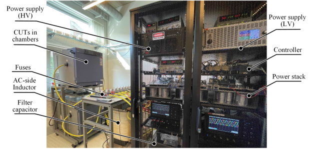
Fig. 3. Photo of experimental test rig.
