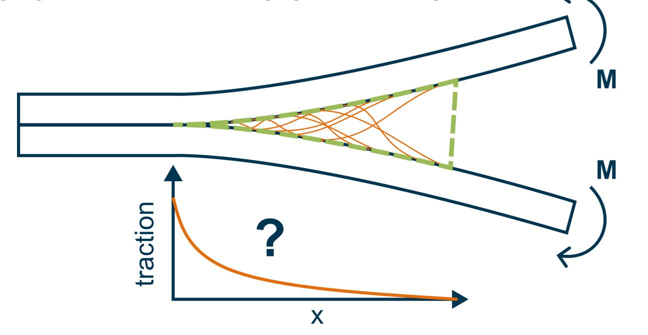
The bridging traction field will be further investigated through a characterisation of the micromechanical behaviour of individual bridging fibres. By monitoring the damage development of individual bridging fibres, the underlying micromechanics behind the traction field will be uncovered.
