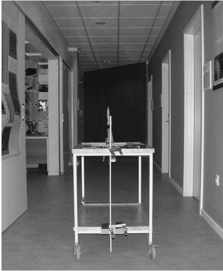
Fig. 4. Handset mounted on wooden stick for free space measurement in the second floor corridor.
