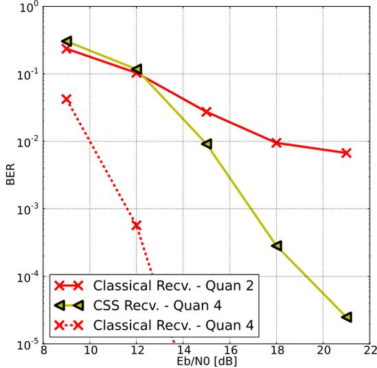
Fig. 6: BER versus  $E_b/N_0$  for a classical receiver and a CSS receiver, both with quantization.  $m = 7$ ,  $S = 10$ ,  $\kappa = 2$  and 100 errors found for each  $E_b/N_0$  point. The dotted line is for a classical receiver with 4 bits of quantization per sample.
