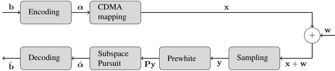
Fig. 2: Flow chart of the discrete numerical experiment.
