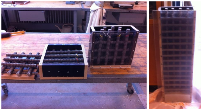
Figure 7 – UHPFRC samples with FiReP®REBAR FRP reinforcement cast at AAU in spring 2012: a) formwork for small samples; b) arrangement of reinforcement in horizontal, vertical and “tall vertical” samples
