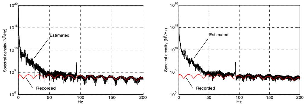
**Figure 8.** Force spectral density obtained using decimation of order 10. 4096 frequency lines.
