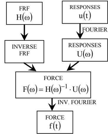
Figure 1. Process to estimate the loading.
