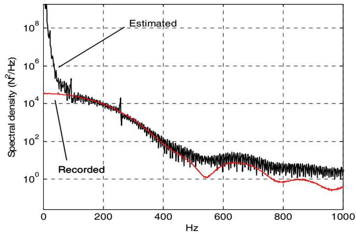
**Figure 7.** Force spectral density at the 8<sup>th</sup> degree of freedom. 4096 frequency lines.
