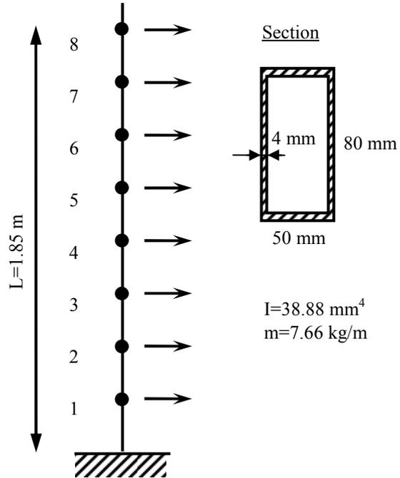
Figure 5. Cantilever beam used in the tests reduction
