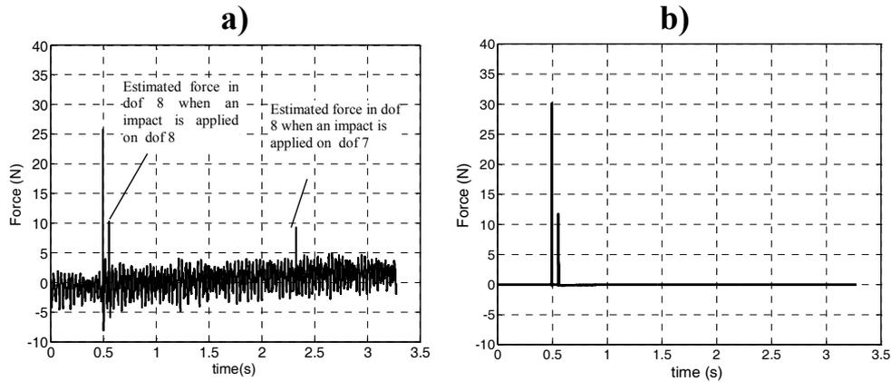
**Figure 9 a).** Force estimated in the 8<sup>th</sup> degree of freedom. High pass filter at 25 Hz. **b).** Force recorded from the hammer in the 8<sup>th</sup> degree of freedom. High pass filter at 25 Hz.
