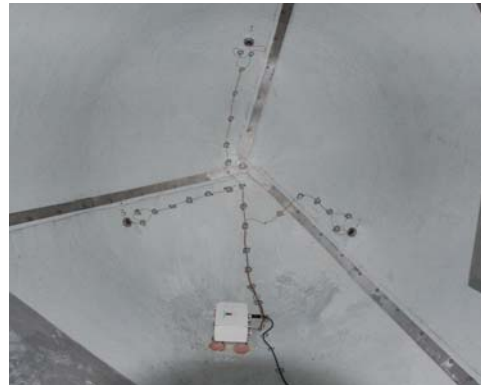
Figure 17 The mounted sensors and the measurement box, seen from the inside of the spinner.
