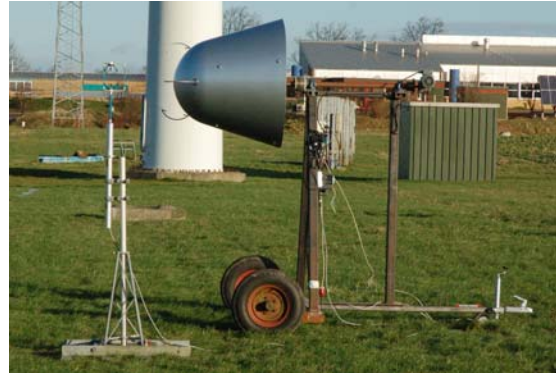
Figure 12 Arrangement of the spinner anemometer comparison with the sonic anemometer at the test station at Risø
