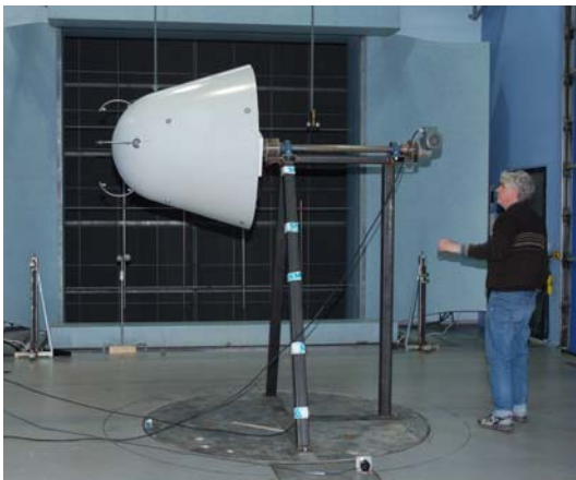
Figure 5 Arrangement for concept tests in a 4 \times 4 \text{ m}^2 wind tunnel. The spinner is seen yawed to -90^\circ and the sonic sensors can be seen on the nose of the spinner. One sensor is horizontal in which position the sensor wind speed was measured with a sweep from -90^\circ to 90^\circ and related to the cup anemometer wind speed measured in the lower left corner of the inlet to the open test section.
