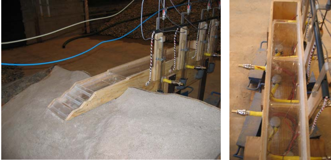
Figure 2. Uncompleted SSG model during the installation in the tank (left), with back compartments equipped with pumps for the measurement of the overtopping rates (right).
