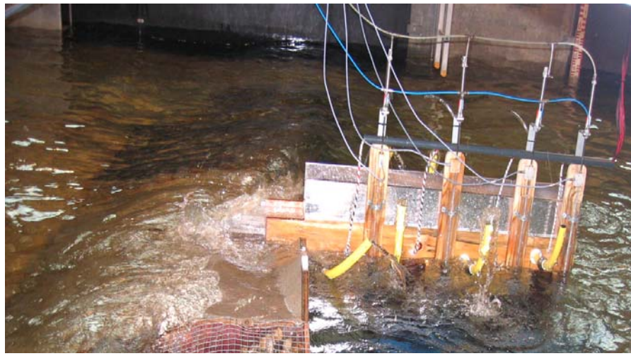
Figure 3. The completed model of the SSG sitting on the reproduction of the cliff at the selected location (above). Under the model during test W3D2S1L0N1.
