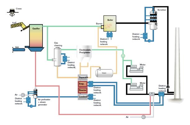
Figure 2. Harboøre district heating plant flow diagram [15]
