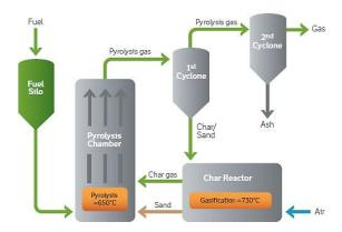
Figure 3. Pyroneer gasifier process flow [21]
