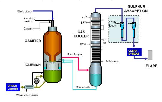
Figure 6. Black liquor gasifier by Chemrec [39]
