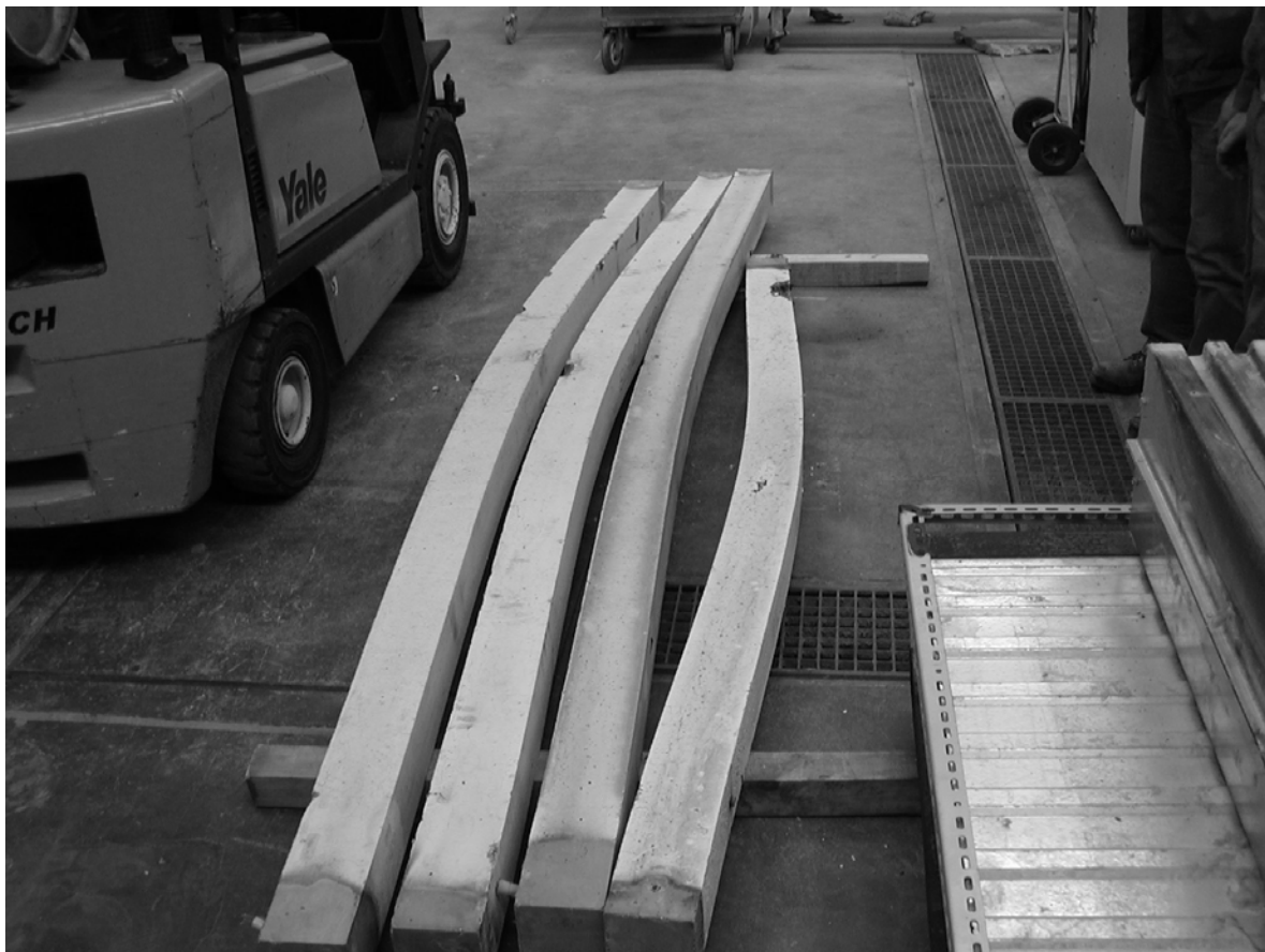
Figure 9 - Some of the columns after fire exposure.
