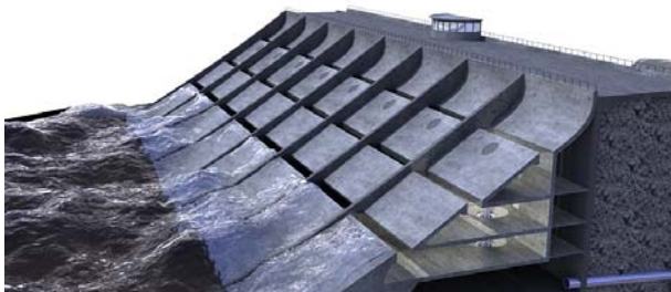
Figure 1 – Artist impression of the Wave Energy Convert (WEC) Seawave Slot-Cone Generator (SSG)
