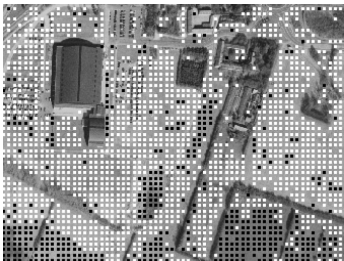
Fig. 4: Division of DTM into two categories: 1 – model was checked and improved, 2 – application of another method is necessary. The division is carried out fully automatically.
